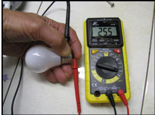
This meter also has the “2K, 20K, 200K, 2M and 20M resistance ranges. These are much higher values of resistance, and would not likely be found in typical stuff around your house.
