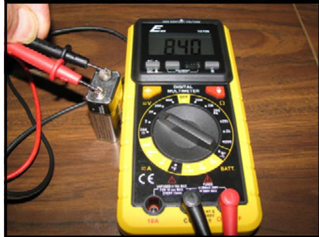
If you’ve got a A123 pack, these batteries will measure about 3.6 VDC per cell, so a two cell battery pack will measure 7.2 Volts DC. Incidentally, if you should accidentally connect a battery to the meter when its set to an AC voltage range, it won’t work. On this meter, it just shows zero volts when connected to a battery.
